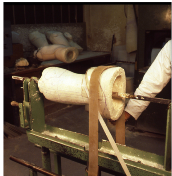
Fig. 52 Thermoforming of polymethacrylate
